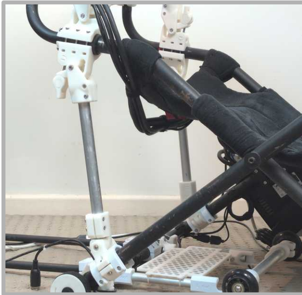
1. Configuration of the side strut for the standard add-on side mount configuration. Requires full Lock-Mod kit.
