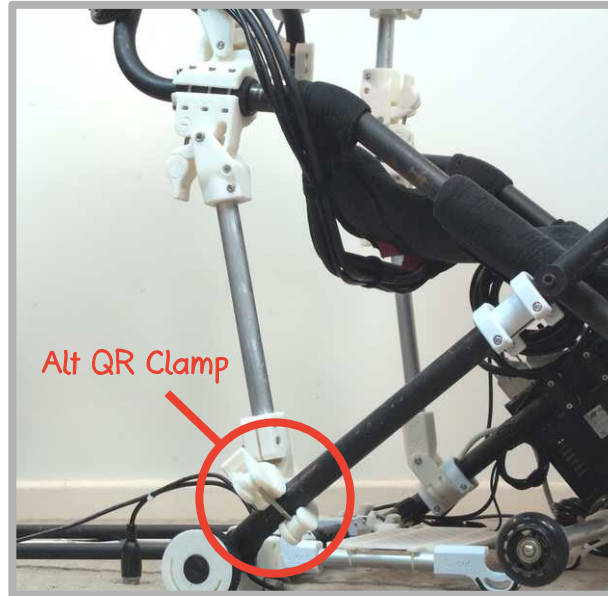
2. Replaces the bottom rotating hinge for a QR clamp to make side strut fully removable. Requires full Lock-Mod kit.
