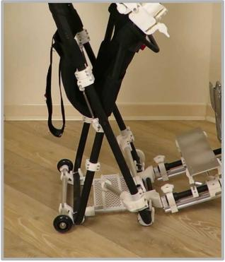
Once the struts have been locked in position, slowly fold and unfold the chair. The struts should feel somewhat 'loose' and free to move around while folding up. If you notice binding or resistance while folding, double check the angle of the struts (ref. previous page) and the alignment of the bump stops.
