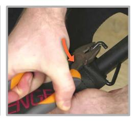
Start by bending the one side of the anchor wire out of the tubing hole. This is best achieved by grabbing the wire along it's length and rotating the pliers. It will take a reasonably large amount of force as the wire is quite thick.
