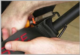
To allow the anchor to be completely removed, bend the anchor wire upwards. The wire needs to be bent far enough to clear the tubing so that the other half of the anchor can be detached from the frame.
