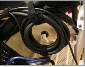
A good place to coil excess cable is just below the seat fabric velcro on the PSC X tubing. Here it doesn't interfere with folding and won't drag along the ground when folded.
