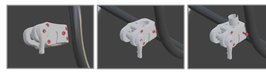
If attaching to the wheelbase tubing, as will be shown in this guide, remove the inner sleeve and unscrew the set screw. These are only needed if attaching this part to the 20mm aluminium tubing of the Side Struts.
