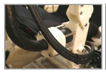
If you want to retain the functionality of opening/closing the wheelbase then any cables going to the wheelbase area should be routed around the outside of the left hinge. If not then outside the right hinge is viable as well.
