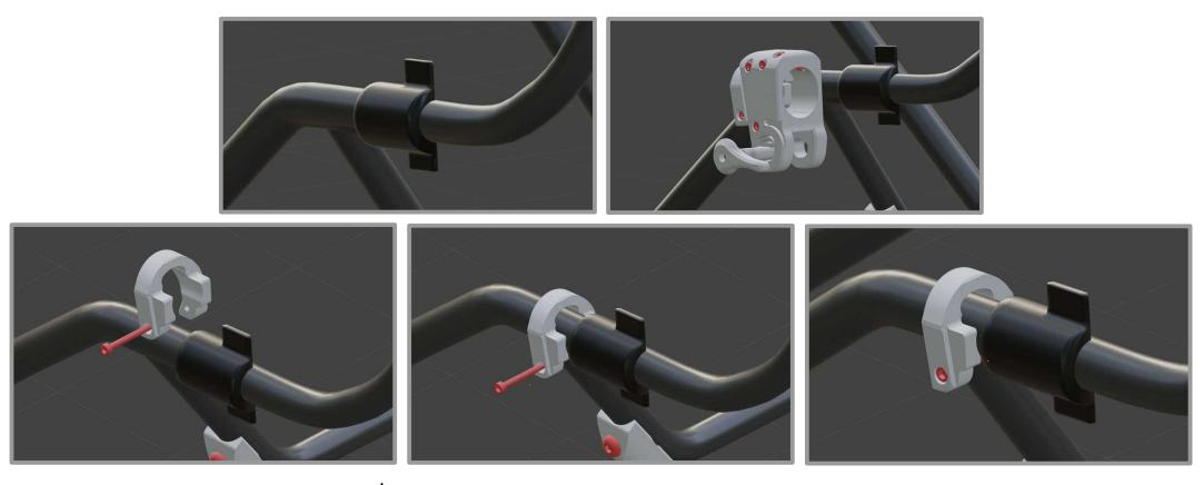
For the right Seat Frame Strut Connector/Reinforcer, remove the small clamp from the main unit and push it on the tubing just behind the black plastic hinge. Once in position the clamping bolt can be loosely threaded back into place.
