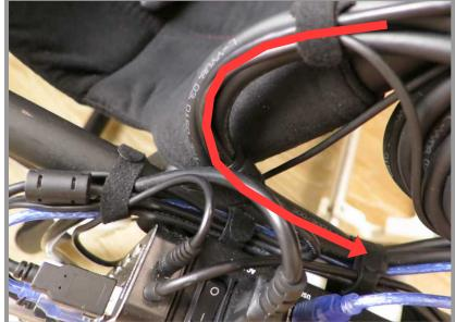
Cable running between the main rig and the pedal tray needs a different approach. Due to the pedal tray extending/retracting when folding/unfolding, a fairly large amount of cable slack is required. The zip tie anchor points shown in the image below gives enough slack to prevent the cable over-extending while also keeping the it from dragging along the ground when moving the folded rig.
