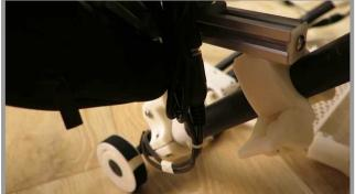
Cables going to the side mount assembly should be routed over the front of the front leg tubing. If routed behind the tubing the cable can be over-extended when the assembly rotates and folds inside of the Playseat Challenge X legs.
