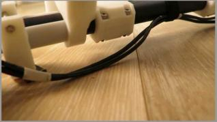
For cables going along the bottom-front tubing, route the cables behind the pedal feet and underneath the roller lock struts, and zip tie in place outside of both front feet and to the middle of the tubing. With a small amount of slack in the cable, this arrangement will allow folding/unfolding without risk of damage to the cables.
