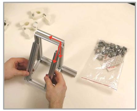
Aim to triangulate the structure when building the side assembly; as much as is possible, each corner of the structure should have 3 profile pieces connected together (or as close to the corner you can get). This provides maximum rigidity and avoids applying excessive bending loads to the right angle joints when loads are applied to the structure.
